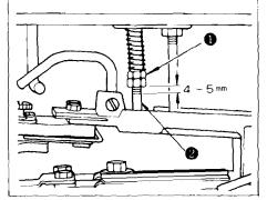
The standard work pressing force is obtained by providing a 4 to 5 mm clearance between the bottom face of nut **1** and the bottom end of the screw of pressure adjusting bar **2**.
