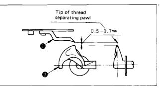
Height of the moving knife thread separation nail
