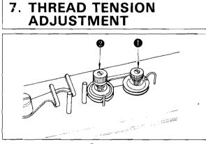
Tension post No. 1 **1** is used to adjust the thread tension to sew on the button and a relatively low tension will be enough. Tension post No. 2 **2** is used to adjust the thread tension applied to the root of the button sewing stitches. This tension must be determined according to the type of thread, fabric and thickness of the button and must be higher than that of tension post No. 1 **1**. Turn the tension nuts clockwise to increase or counterclockwise to reduce the thread tension.
