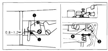
Provide a 0.8 to 1.2 mm clearance between nipper 1 and nipper block 2 to prevent the nipper from nipping the thread while stitching. Loosen screw 3 and move nipper bar block 1 to the left or the right.
