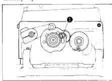
★ 8 stitches (6 stitches) Pull stitch adjusting cam knob ● and set it as shown in the illustration.
