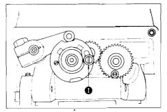
★ 16 stitches (12 stitches) When stitch cam knob ④ being set for "8 stitches" has arrived at the right end as illustrated, set knob ● in the illustrated position.
