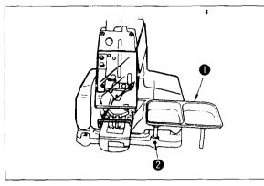
Insert the posts of button tray ① in hole on the right of the machine sub-base and tighten each setscrew ②. You may use also the installation hole on the left if the operator wants.
