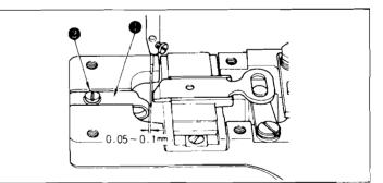
Loosen screw @ and provide a 0.05 to 0.1 mm clearance between the needle guide ① and the needle by moving the needle guide ① to the left or the right when the needle is in the lowest position.
