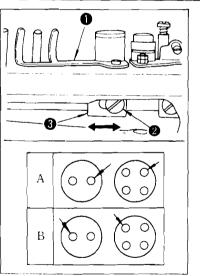
Adjustment of the thread pull-off lever ①, insert a screw driver through an opening in the machine arm side cover (left), loosen screw ② and adjust the position of nipper bar block (rear) ③ to the left or the right.
