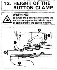
The standard clearance the between the bottom face of button clamp jaw lever and the top face of feed plate is is 12 mm for MB-373 and 9 mm for MB-373. Loosen screw and adjust the height of button clamp lifting hook (1).
