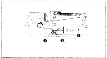
\* Clearance between the button clamp lifting lever and the adjusting screw
