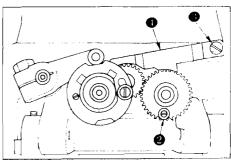
\* 32 stitches (24 stitches) When the number of stitch is set to 16, move stitch number adjusting gear roller 2 to the lower position. Now, attach stich number adjusting lever 3(optional) in position using screw 3 (optional).
