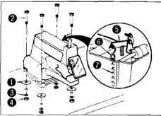
Put rubber cushion ① on the table, place the machine head on the rubber cushion and fix it to the table using screws ②, plain washers ③ and nuts ④. Attach "S" chain hook ① and chain ⑦ to stop motion trip lever ⑤.
